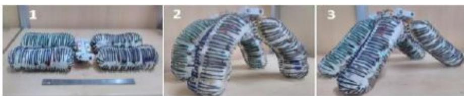
Fig. 1: Quadruped incorporating CObRaSO module in [1] Crawler configuration, [2] Legged configuration, [3] Wheeled configuration;
