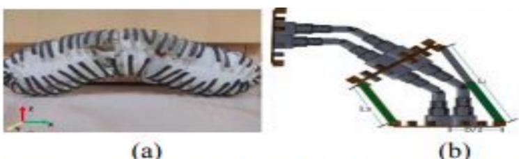
Fig 4: (a) Prototype of the module in the bend configuration. (b) The telescopic screw based 3-DOF manipulator achieving bend configuration.
