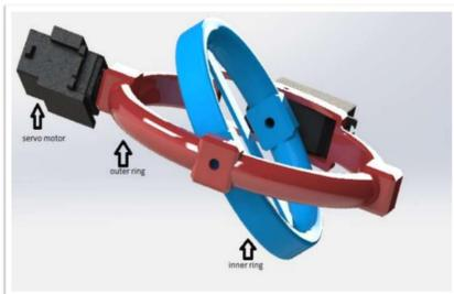
fig 1. Gimble mechanism.
