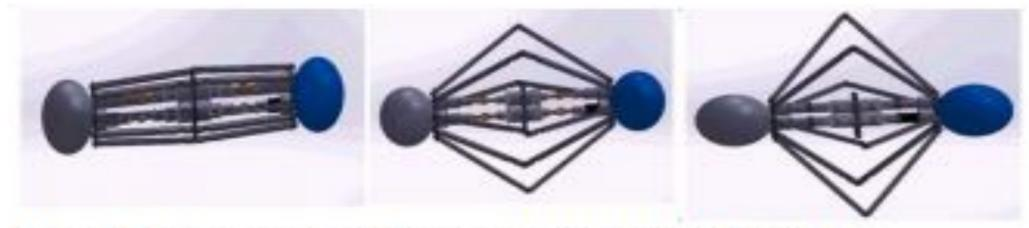
Fig 3.: The transformation from crawler to spiked-wheeled mode.
