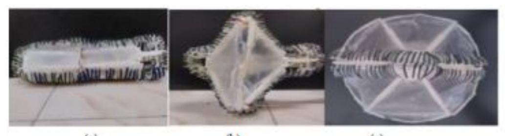
Fig. 2: Transformable compliant Omni crawler robot, (a) Elongated Crawler mode, (b) Transformed wheeled mode side view, (c)Transformed wheeled
