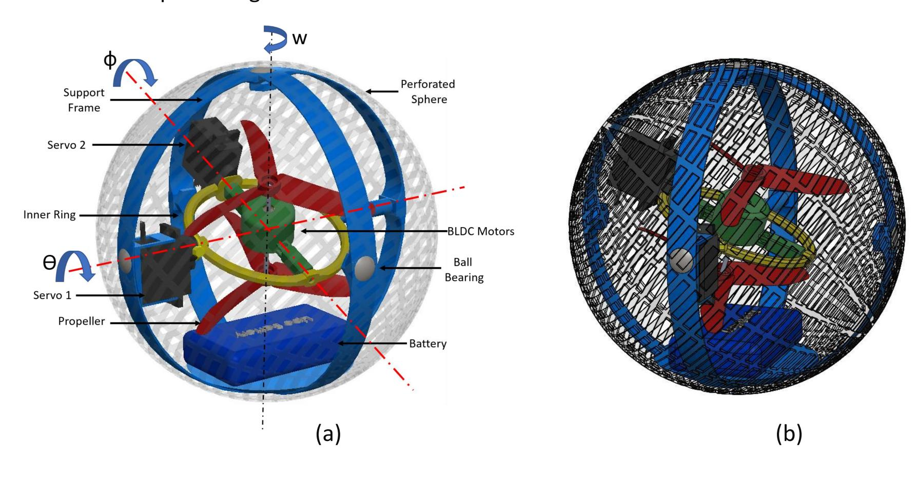
Figure 3. (a) Mechanical design of the OSWalT consisting of two servo motors and inner ring forming gimbal mechanism (b) Final model of OSWalT.
