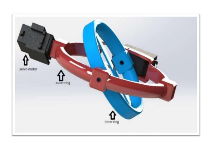
fig 1. Gimble mechanism.
